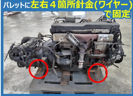
firmly attached to the pallet with wires
